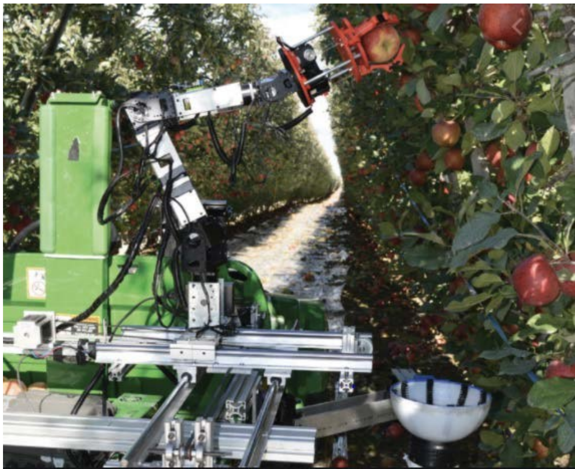
Figure 7: Robotic picker harvesting apples grown on a crop support structure (only trial phase).
