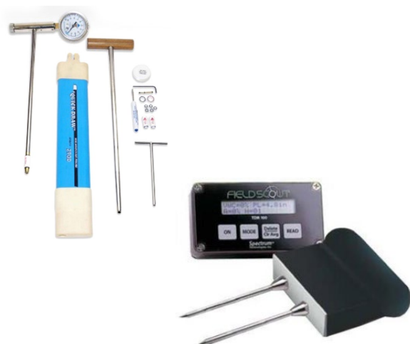
Figure 5.1: Examples of soil moisture probes. Left - Quick draw tensiometer. Right - Hand-held time-domain reflectometer.
