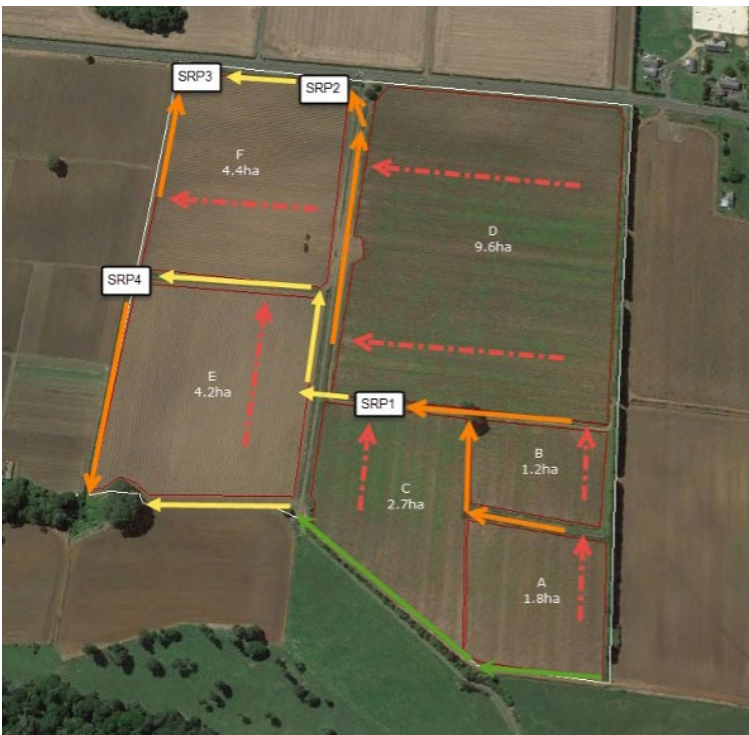
Figure 2.1: A simple digital map with drawn features to show drains and flow of water.
