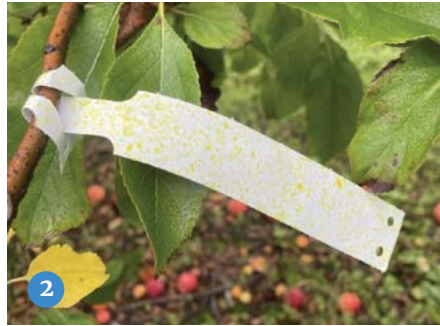
1 Water sensitive papers turn blue when spray droplets come into contact and are a good tool for evaluating spray coverage, 2 Yellow dye tracer was used to measure how much spray was deposited on leaves or 'artificial leaves' (plant tags), 3 Samples were rinsed in water to extract the dye then measured on a spectrophotometer
