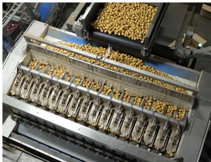
High speed weigher and bagger from Manter
