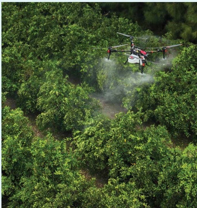
Drones can better access older, densely planted trees with closed canopies where a tractor cannot get through
