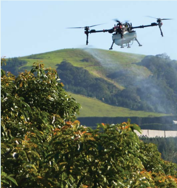
Penetrating the dense foliage of a full-canopy avocado tree requires deliberate attention to flight speed, height, droplet size and other factors
