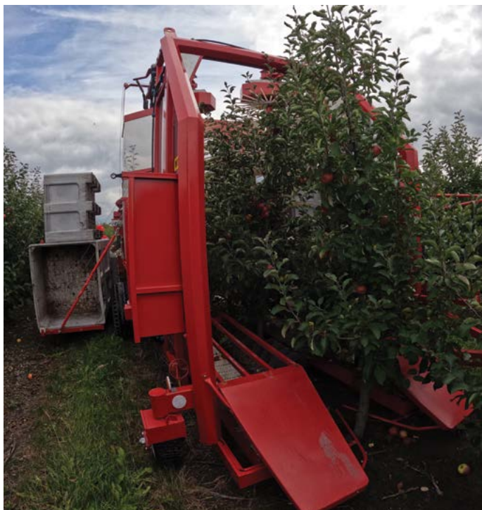
The premium cider roadmap report describes the benefits of mechanisation such as the Polish Weremczuk tractor-towed harvester. Source: Weremczuk Agromachines
