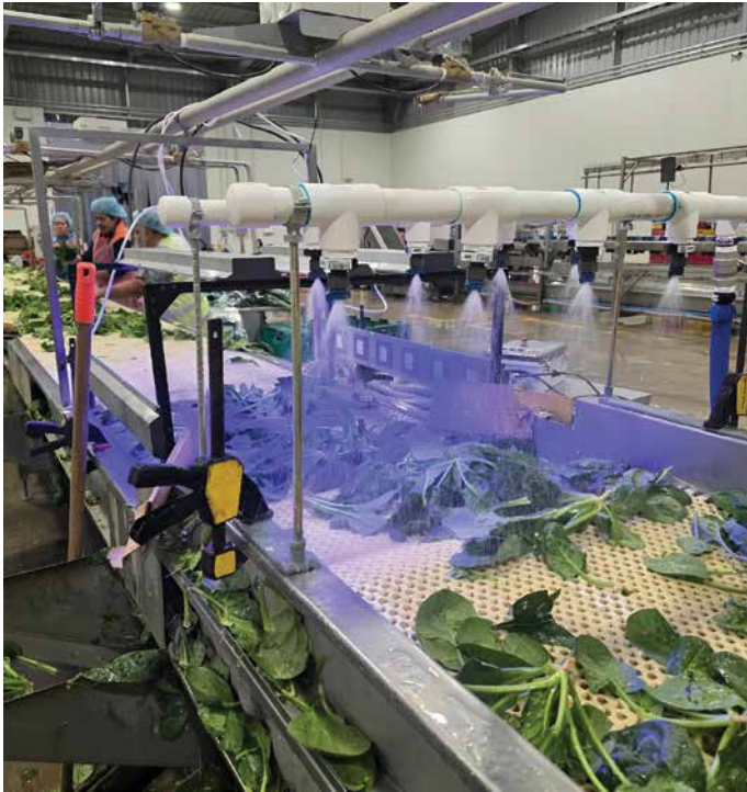
Plasma activated water system and dual light unit on the conveyor treating spinach during trial
