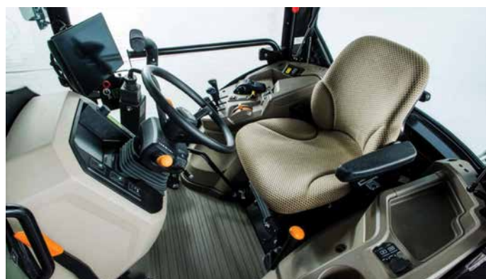
The 5EN cab includes a new digital dash display, an enhanced right-hand console, USB-C ports for modern connectivity, an Electro-Hydraulic (EH) Hitch and an integrated armrest for ergonomic support
