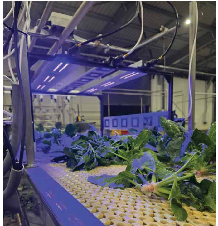
Dual light prototype on the conveyor treating spinach during trial
