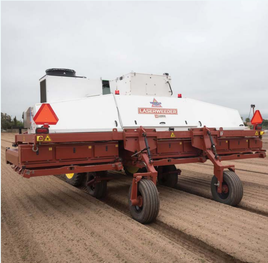
The LaserWeeder zaps weeds and leaves crops untouched. Photo courtesy of Callaghan Innovation
