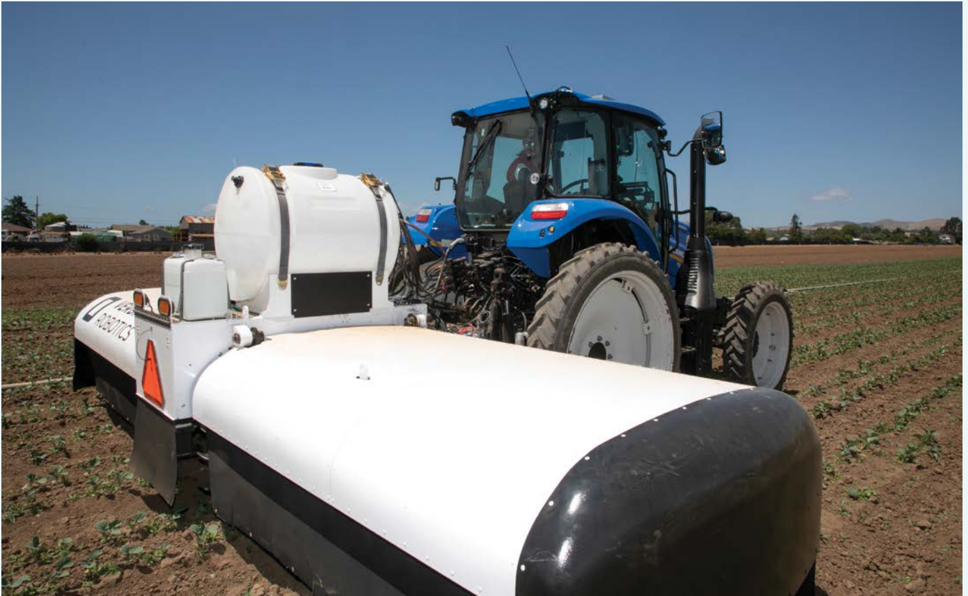
Verdant Robotics from the United States manufactures a spot sprayer that identifies weeds and avoids blanket spraying. Photo courtesy of Callaghan Innovation
