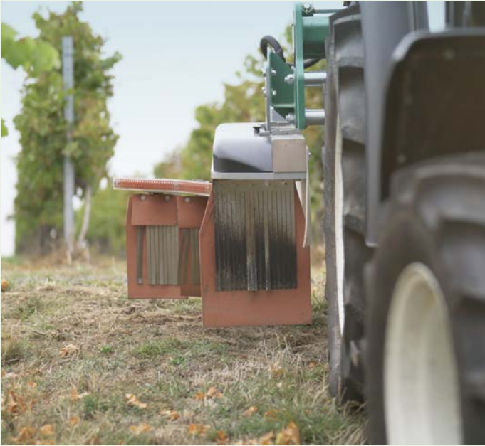
The high voltage (5000-15,000 V) heats the water in weeds to boiling point so they explode from the inside out. Photo courtesy of Zasso Group AG
