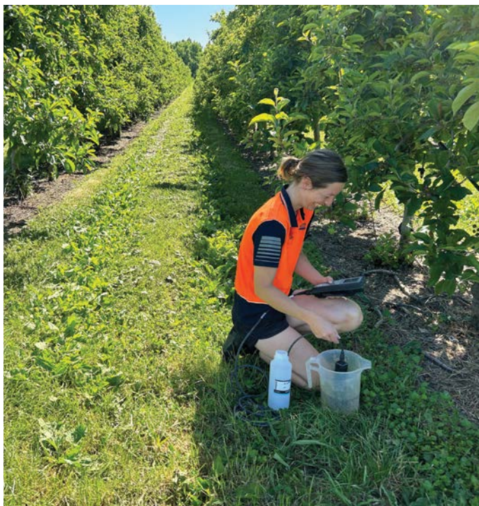
A technician measuring the pH, temperature, dissolved oxygen and conductivity of water from the tile drainage in an apple orchard
