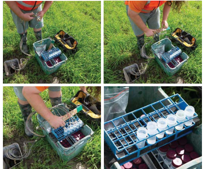
Figure 3: Collection of leachate samples from the ryegrass crop in Hawkes's Bay. Clockwise from top left figure: placing vacuum on suction cups at 60 cm and 120 cm soil depth to extract soil solution. Vacuum is placed on the suction cups for 1 hour. Tubes are identified depending on depth and prepared to release suction. After suction is released, solution flows into the collecting vials. The last image shows the vials with soil solution samples. Vials are then sealed and frozen until laboratory analysis can be completed
