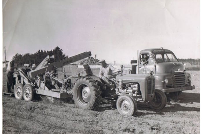
Jac Bleeker on a tractor pulling the wooden potato harvester he built, which was one of the very first bulk handling potato systems in New Zealand
