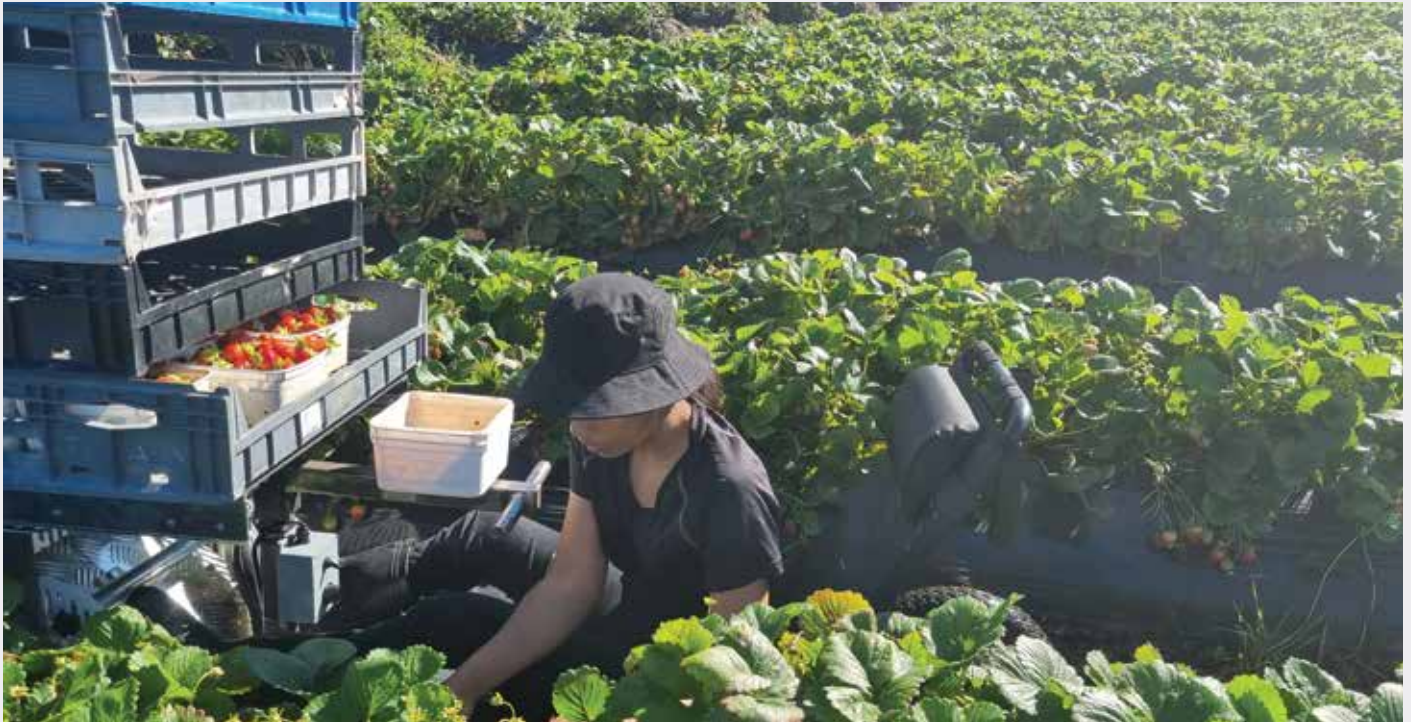
The e-Bin modular robot developed at the University of Waikato towing strawberry pickers in a harvesting buggy – the modular solution can be reconfigured to assist in kiwifruit harvesting and orchard activities to ensure year-round utilisation
