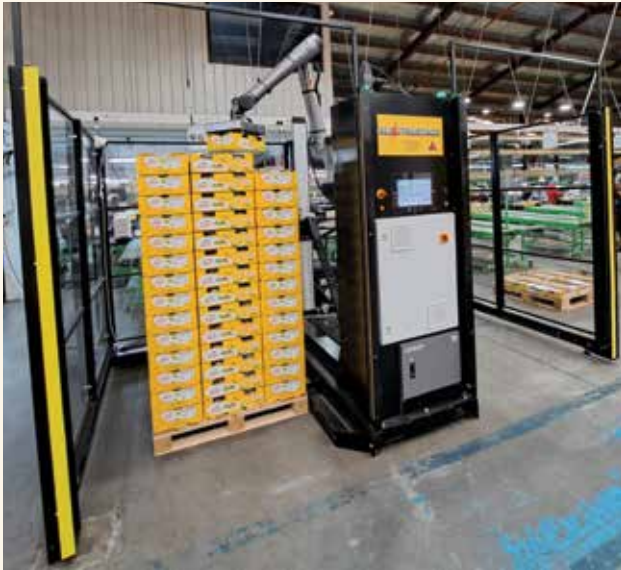
Electrostack's robot palletiser in action during a trial at Seeka packhouse in Te Puke
