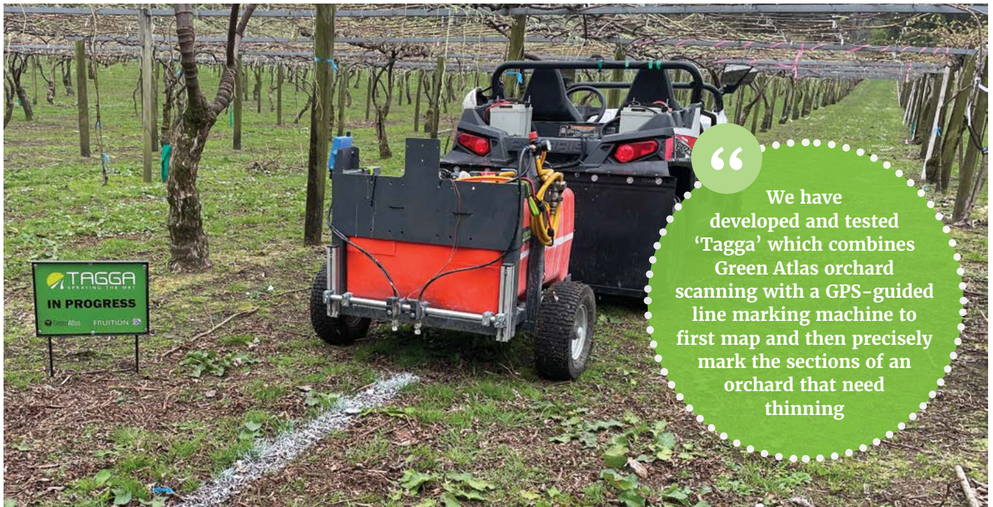
A GPS-guided line marking machine precisely marks the orchard sections that need thinning
