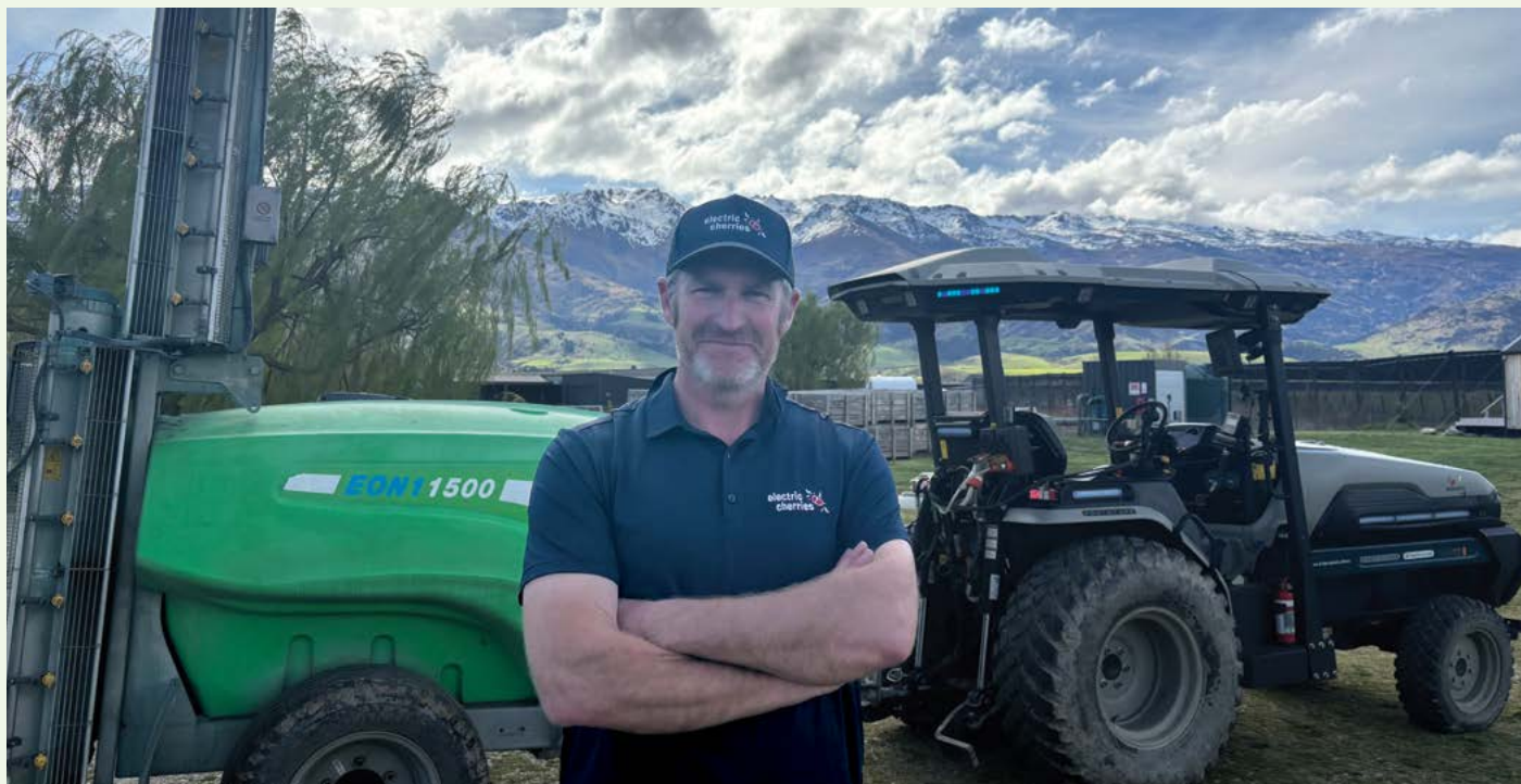
The Californian Monarch electric tractor with its New Zealand-made sprayer has a spray runtime of 10 hours
