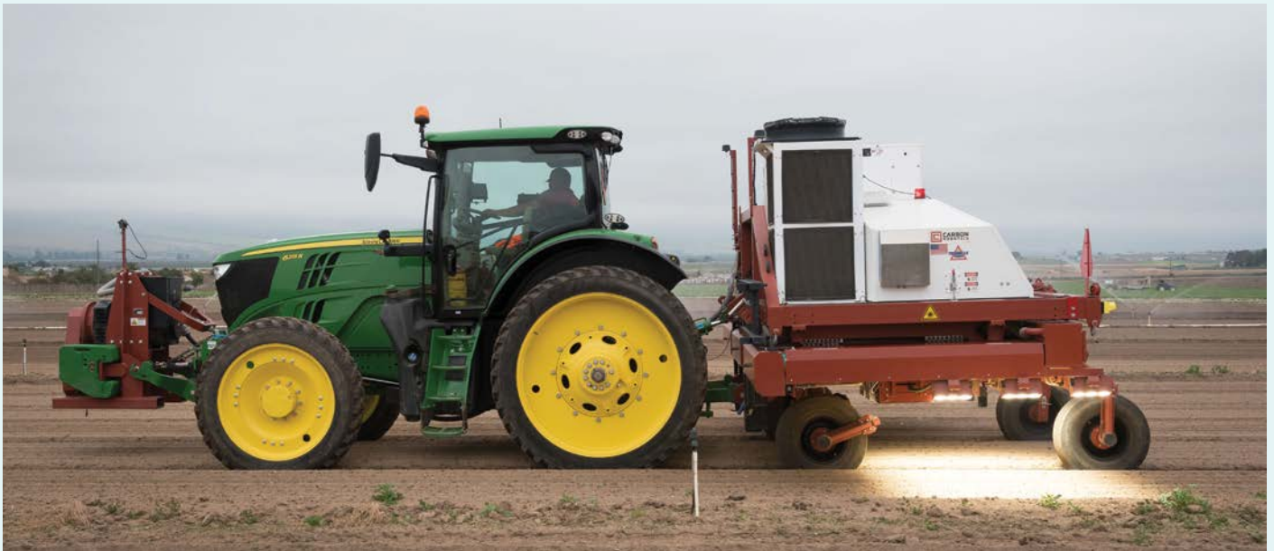
The laser weeder by Carbon Robotics recognises and eliminates any type of weed without touching the crop
