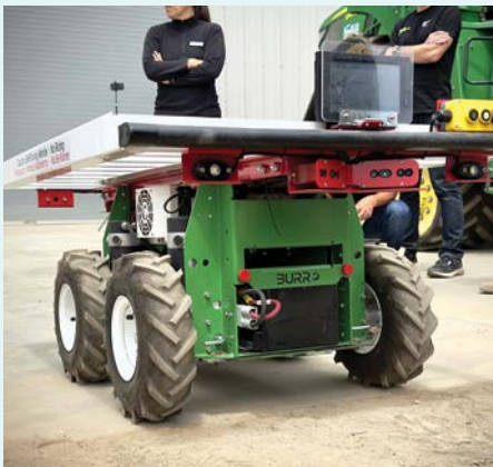
"Burro" is a smart robot platform designed to follow people and navigate autonomously
