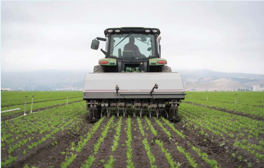
The mechanical weeder by Stout Agtech intelligently recognises the crop, its blades opening and closing around the plants as it goes along the bed
