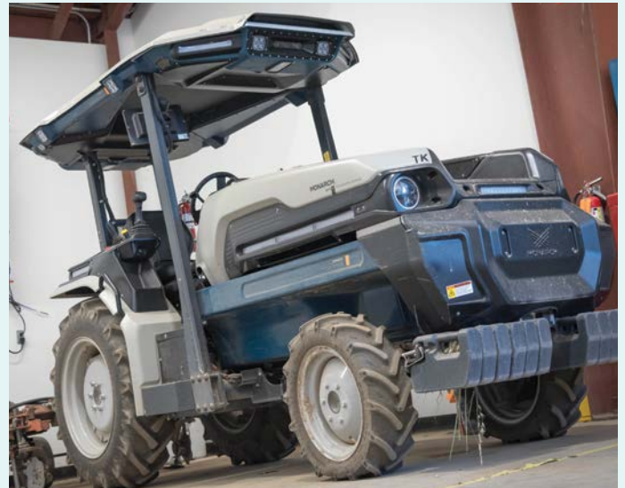
Monarch MkV tractor used for discing and mowing in a vineyard: one of several autonomous platforms available commercially
