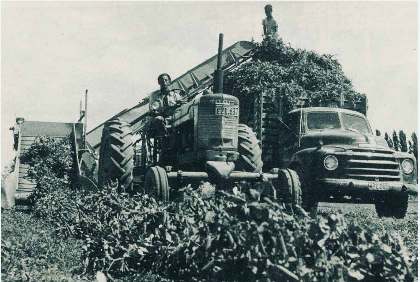
A tractor-drawn loading elevator, driven by Stan Cooper, filling a truck, while loader-boy Guy Dods attends to stacking the vines
