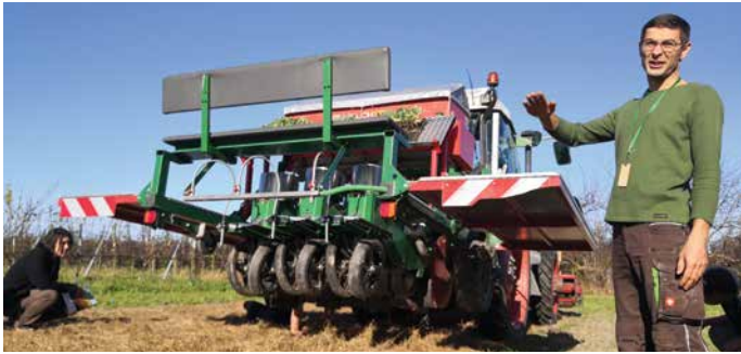
Tobias Euerl demonstrating the live2give MulchTec Planter, designed to transplant seedlings through thick mulches or straw
