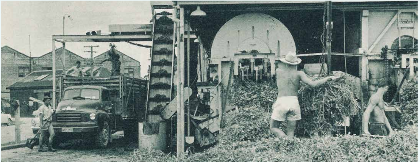
Feeding the peas into viners, while the waste is discharged into a truck to be used as silage
