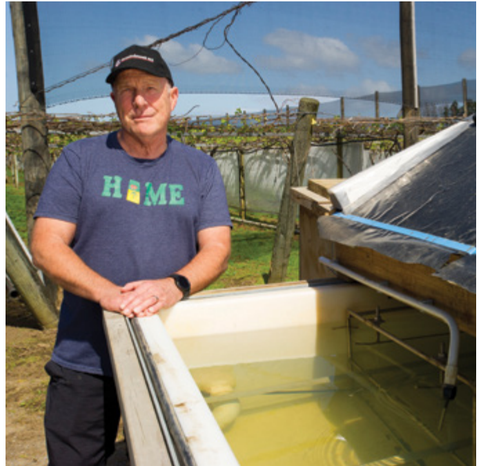
Bruce Rapley with a self-designed hot water bath to control cyclamen mite. It operates at a specific temperature of 44.4°C
