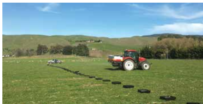
Calibrating a broadcast spreader with a set of fertiliser catch trays in the paddock. Enter details and weights into FertSpread to have calculations done and a report generated.
