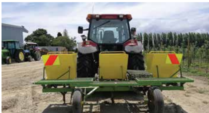
Side-dresser ready for calibration using the FertSpread.nz bucket test for placement equipment. Enter details and weights into FertSpread to have calculations done and a report generated.
