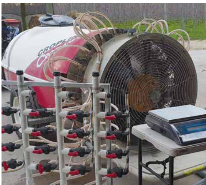
Detailed calibration of an orchard sprayer. (Photo Andy Mawley, Fruition Horticulture.)
