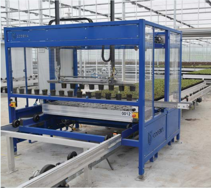
Superb Herb's robotic system automates the process of spacing the seedlings out onto an ebb and flow table
