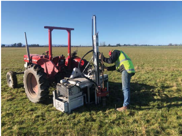
Collection of deep soil cores for soil bulk density analysis. Bulk density is used to scale laboratory results expressed in units of mg N/kg to field scale results in units of kg N/ha. Don't panic - this level of testing will not be required when using the SVS tool
