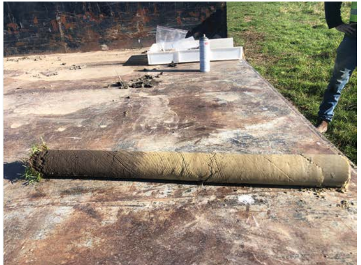
Collection of deep soil cores for soil bulk density analysis. Bulk density is used to scale laboratory results expressed in units of mg N/kg to field scale results in units of kg N/ha. Don't panic - this level of testing will not be required when using the SVS tool
