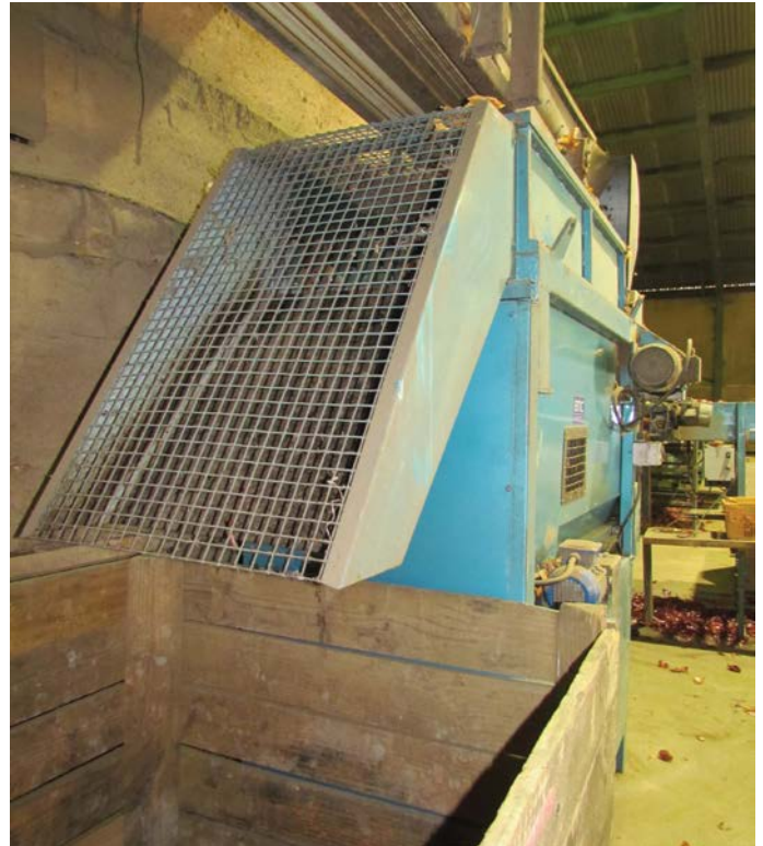
The extended guards now prevent a worker reaching up and into the scroll topper hopper
