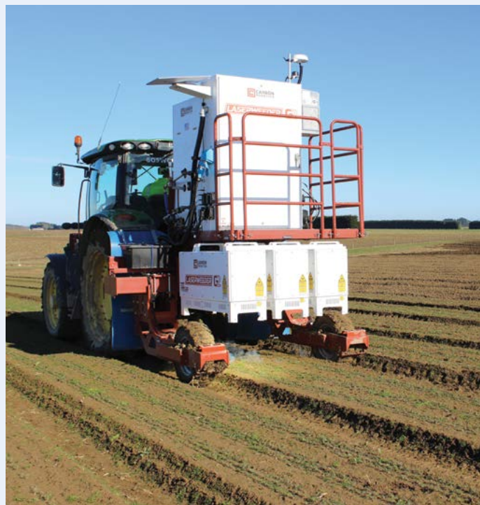
Bright lights and puffs of smoke come from the weeder as it works along the carrot rows. The top two thirds contain coolant for the lasers, above which is the Starlink aerial
