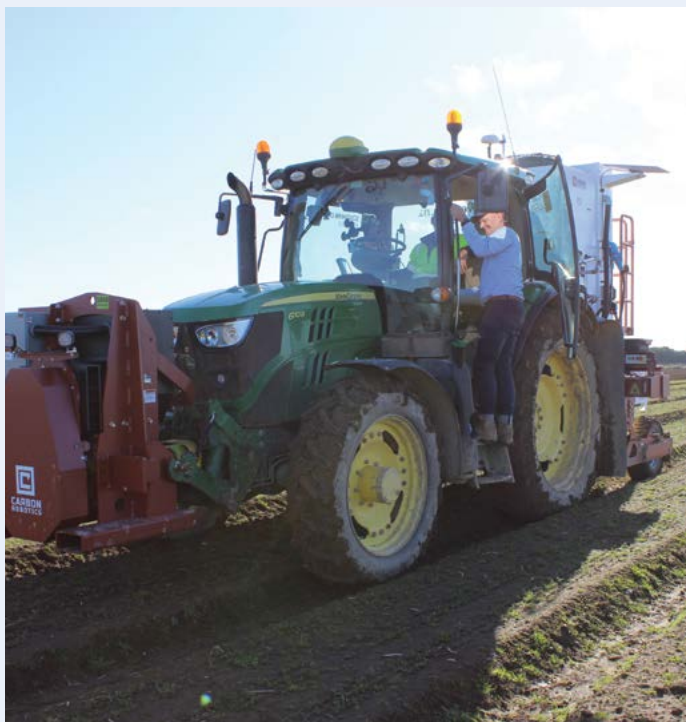
Matthew checks in with the operator of the laser weeder. Note the weeder's generator on the tractor's front PTO
