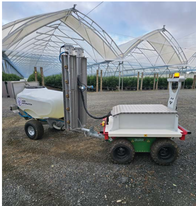
The United States-built Burro Grande with Agri Automation AutoSpray’s 500 foliar sprayer working amongst blueberries in New Zealand
