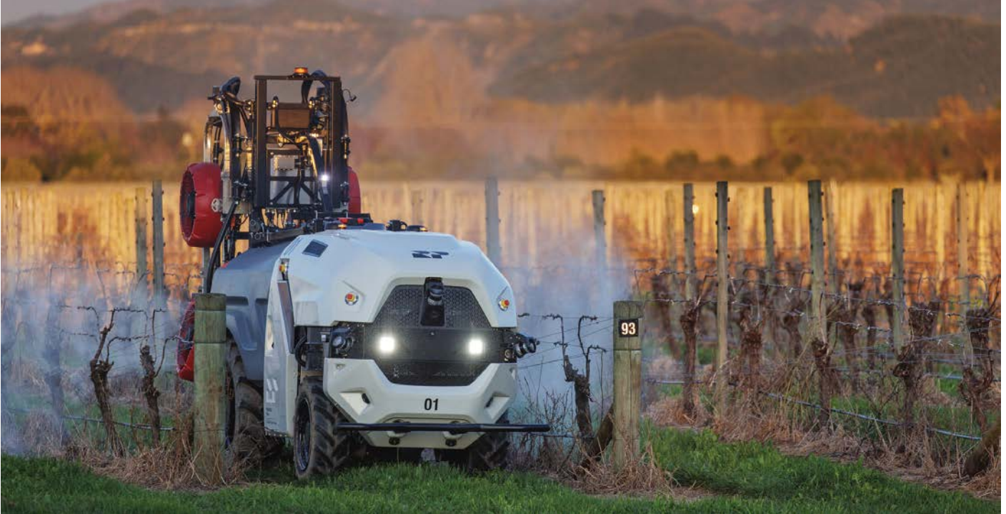
Prospr, distributed by Croplands, at work in a New Zealand vineyard. The autonomous sprayer is designed and built by Robotics Plus in Tauranga
