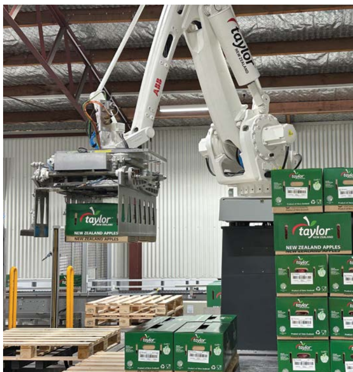
ABB articulated robots deliver high-speed, safe and precise pallet stacking
