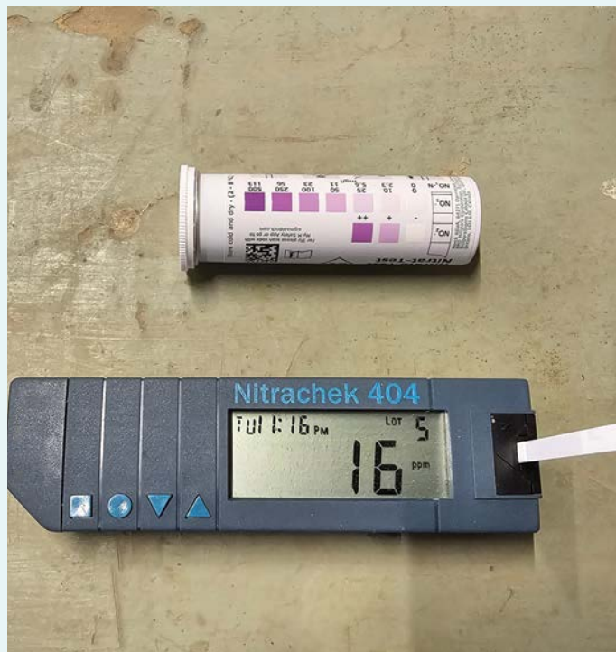
The Nitratechek device gives precise readings of nitrate concentrations measured by Quick Test strips. The LandWISE calculator ensures these readings are accurately converted to kg N/ha for nutrient balances and determining fertiliser rates
