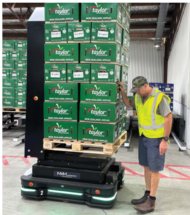
Driverless forklifts reduce visibility-related hazards when operating around people
