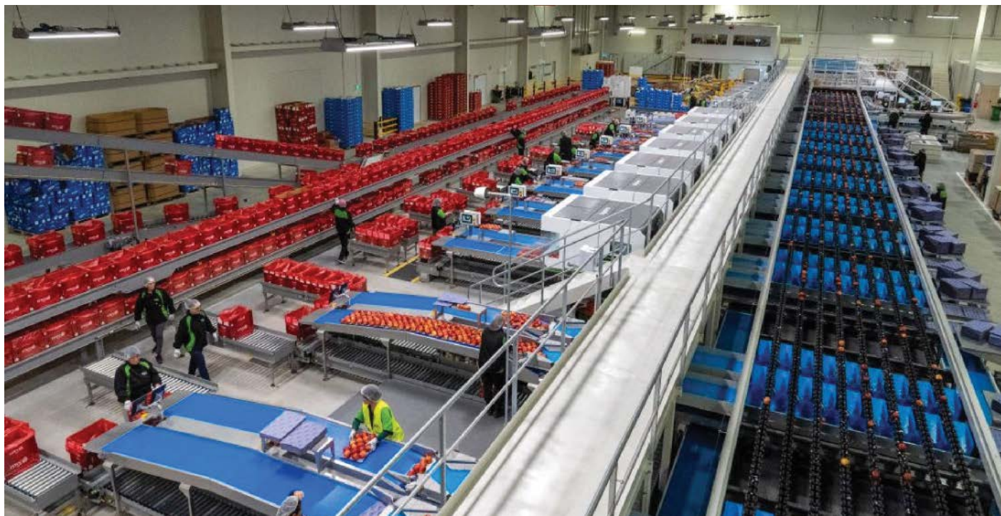
The first-phase 100-metre packing line at T&G's Whakatu facility can process 3000 to 4000 apples per minute
