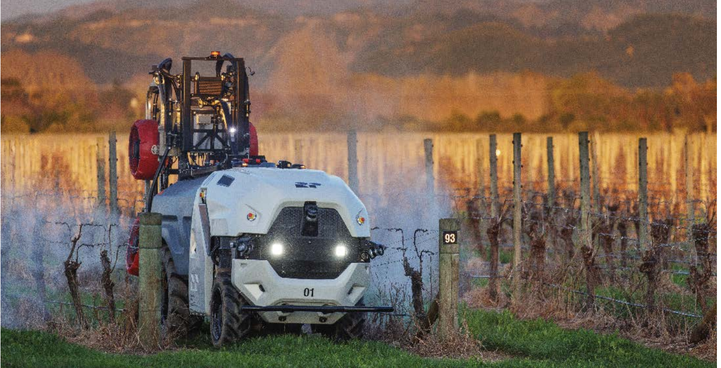
The Q4 / Q6 sprayers, developed by Robotics Plus in conjunction with Croplands, have two or three fans per side. The series also includes a Q8 sprayer with four fans per side, and is best suited to tree crops
