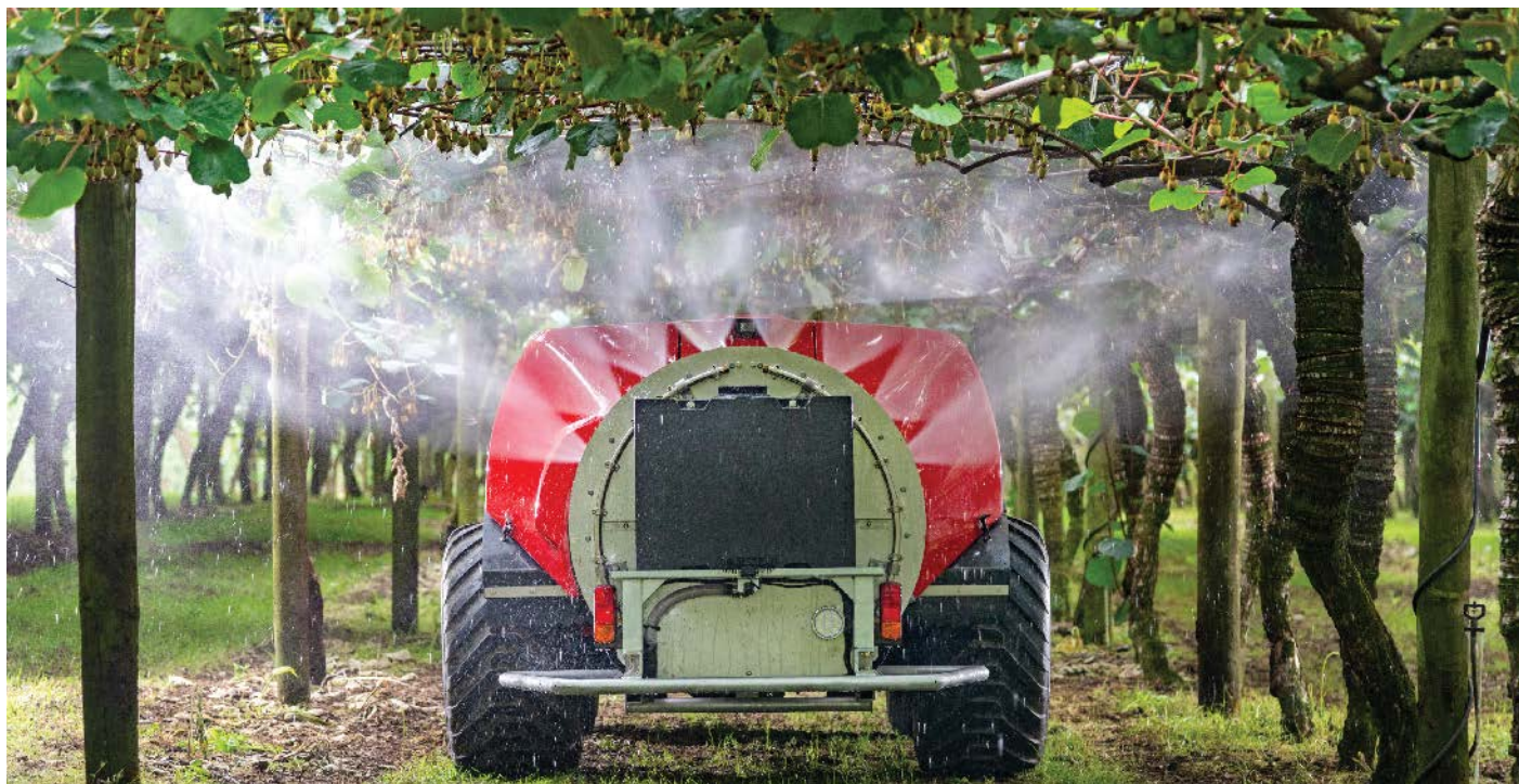
Once the crop canopy has developed, almost all of the applied spray can be expected to land on target. Photo of Cropliner Rover Self-Propelled sprayer courtesy of Croplands
