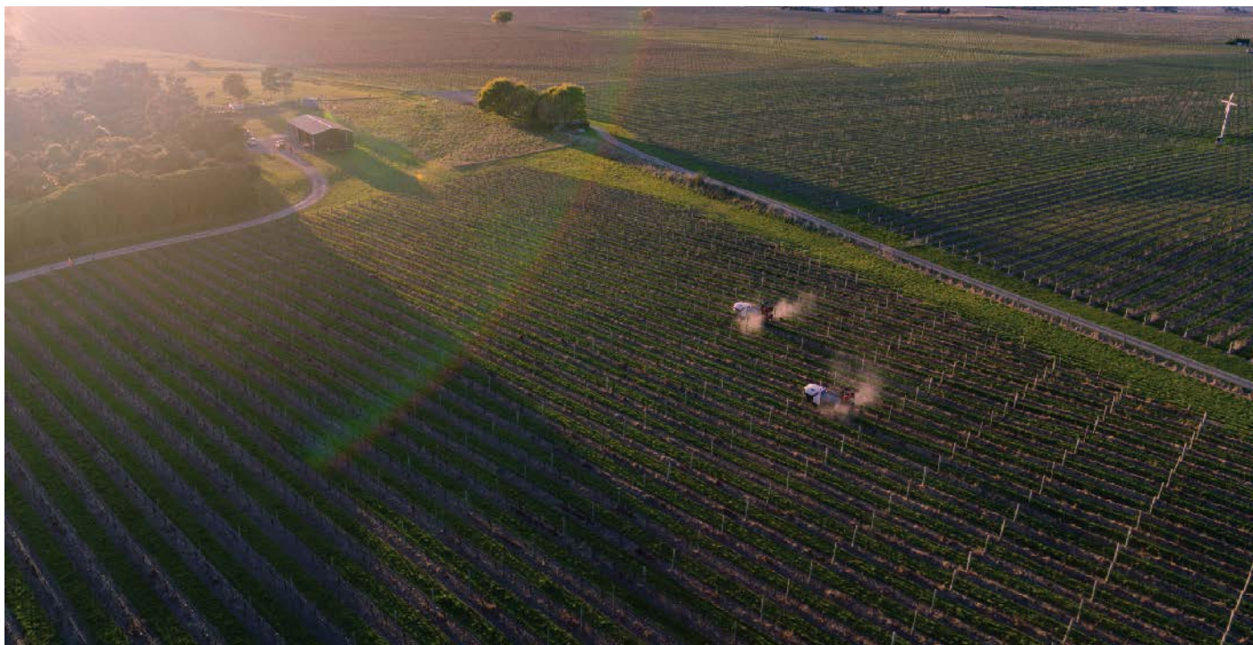
With a spray trial on this vineyard, the autonomous vehicles can turn on their rear axle with a minimum headland requirement of 7.1 metres for row-to-row turning. Minimum row spacing is 1.85 metres
