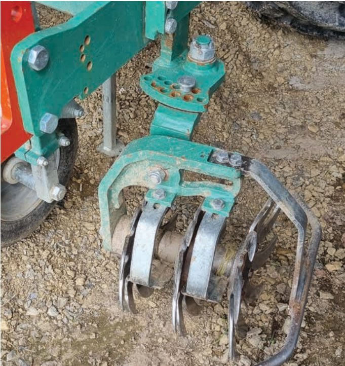
A local viticulturist provided a row hucker tractor attachment to get close to the trees as needed
