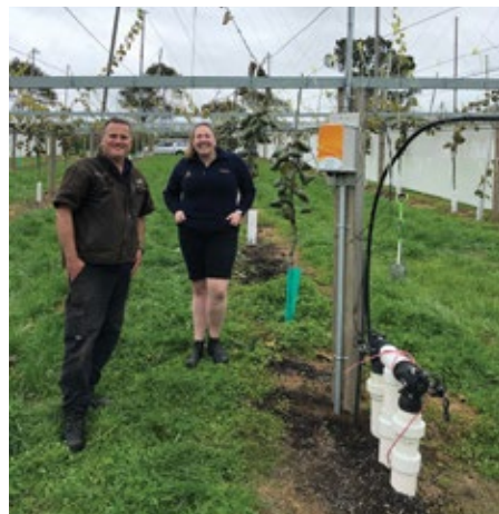
Installed AquaCheck soil moisture probes on Halo telemetry in the Bay of Plenty as part of an integrated block-wide monitoring and control radio-mesh network.
