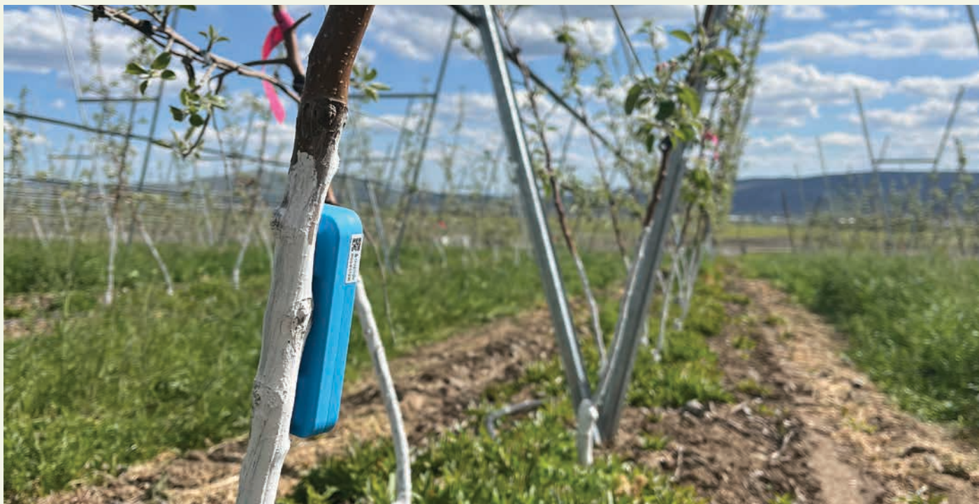
The Croptide device attaches directly to plant stems to analyse and assess the plant's hydration
