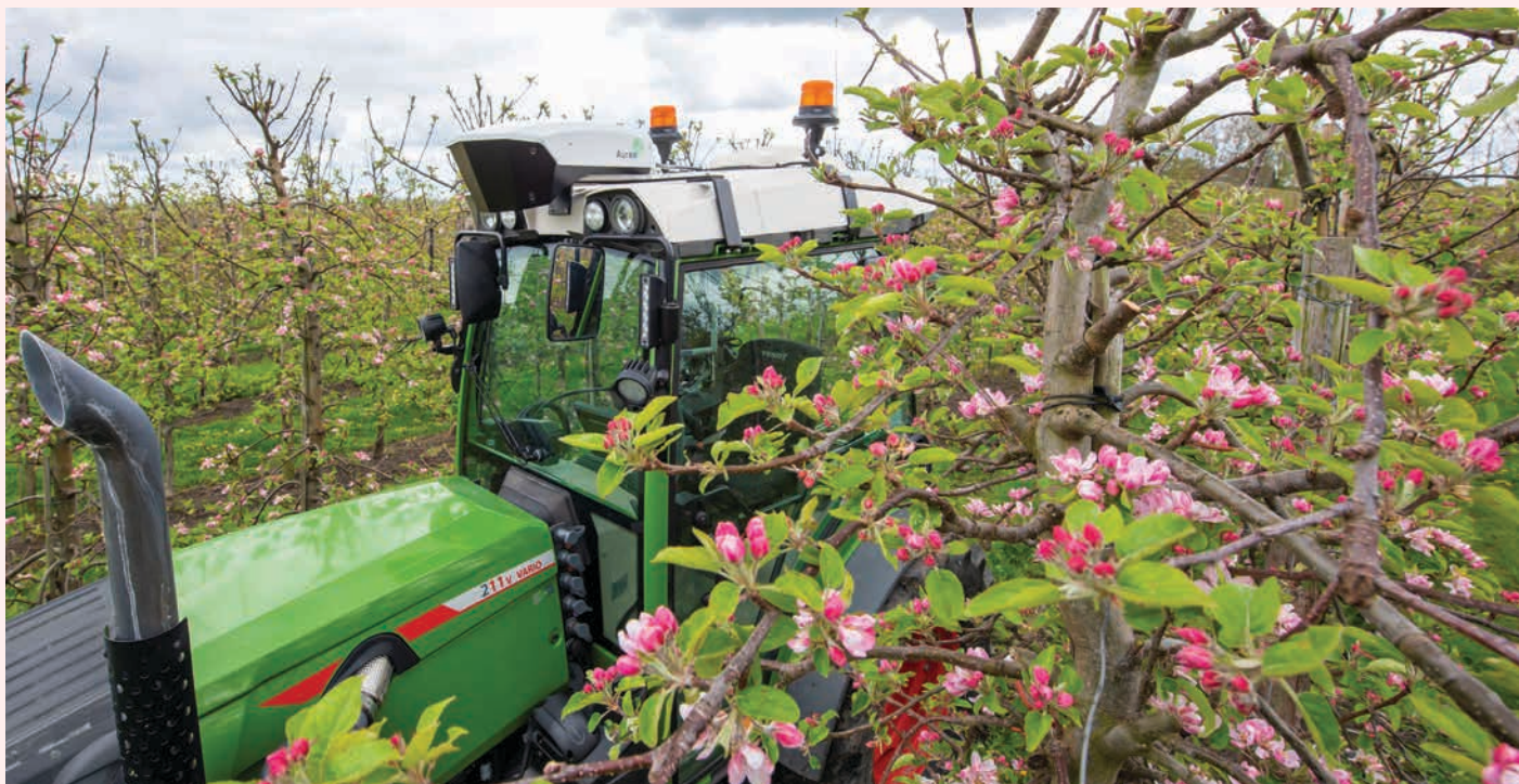
An orchard tractor fitted with Dutch company Aurea Imaging's TMS TreeScout sensor, updating fruit counts, size and canopy development maps every time the orchard is mowed or sprayed
