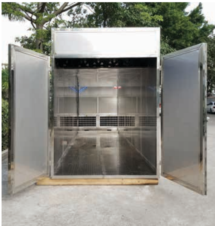
IKE AIO-2400 dehydrator internal view
