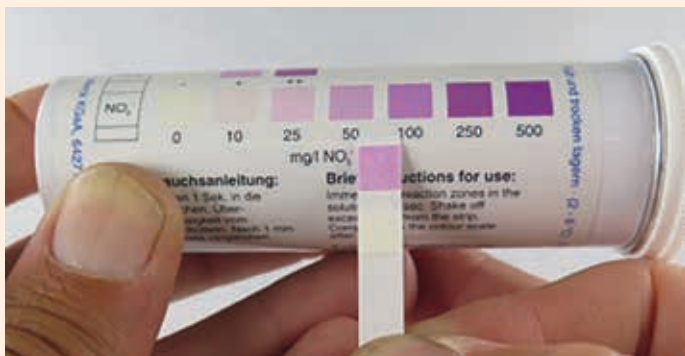
Figure 1 The Nitrogen Quick Test Strip, image from MPI SFF project Nitrogen – Measure it and Manage it
