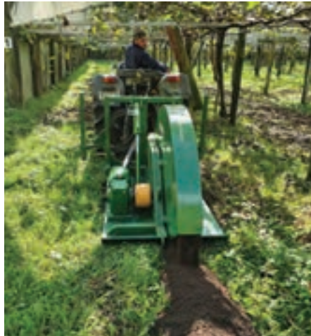
RTS500 Rootsaw under the vines
