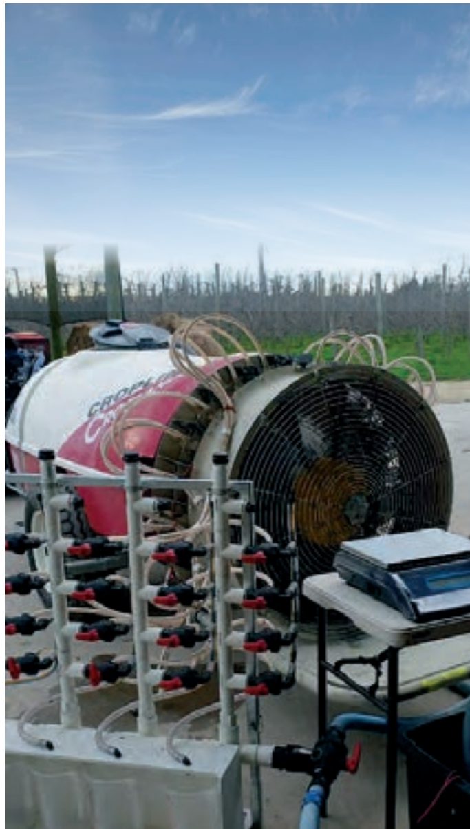
Detailed calibration of an orchard sprayer
