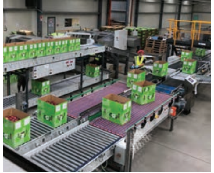
ABC Software provided an integration solution for CAJ van der Voort packhouse's Dutch 14-lane Greefa Geosort system, which can produce about 2,500 cartons an hour.
