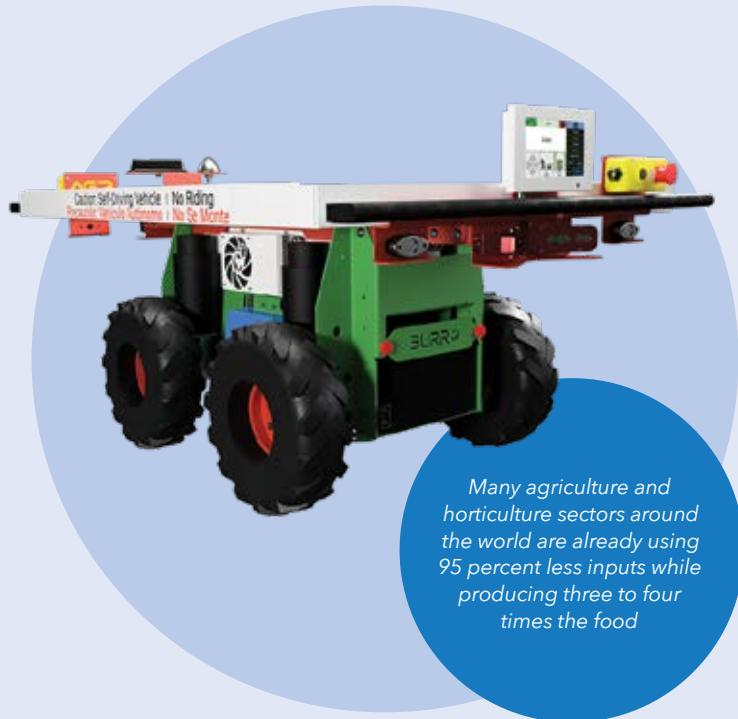
*The Burro platforms use computer vision, high precision GPS, and AI to follow people and navigate autonomously while carrying payloads*
