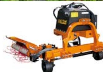
The Berti Ecosprint has a patented rotor with 8m of nylon per spool, which can be easily extended when worn, and will tackle the harshest of weeds without damaging the trunks or plants.
