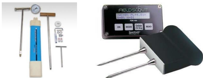
Figure 6.1: Examples of soil moisture probes. Left - Quick draw tensiometer. Right - Hand-held time-domain reflectometer.
